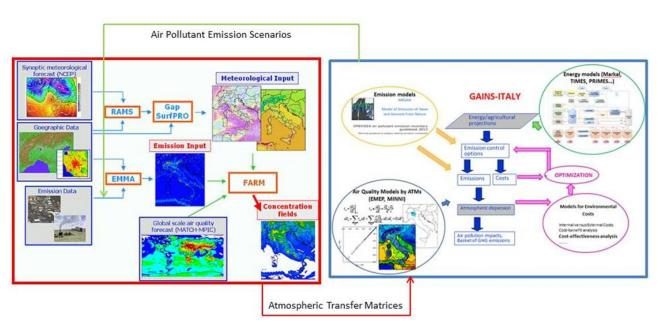
Figure 9.1 – The simplified functional flow-chart of the MINNI national modelling scheme.
