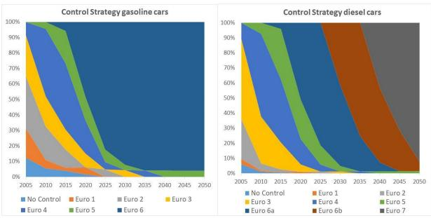
Figure 9.4 – Control strategy for gasoline (on the left) and diesel (on the right) cars.
